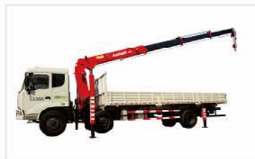
Truck Mounted Crane
